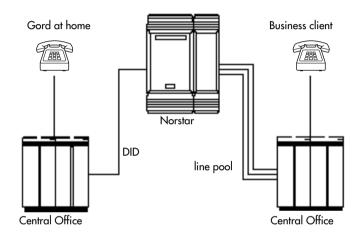
**Hardware:** ICS, a Trunk Module with a DID Trunk Cartridge or DTI with several DID lines
