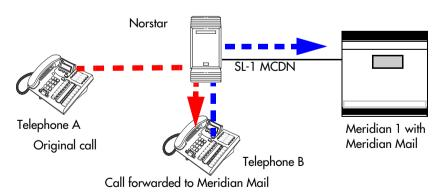
If you are using the centralized voice message system from a Meridian 1 system, you require the following programming on the M1:
